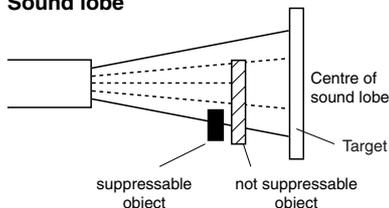
The suppression of the disturbing target is effected through reduction of the response sensitivity. This figure shows its effect on the response characteristics of the sensor. The sensor is preset on step 1 by the manufacturer.
